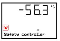
Alarm indication (example: safety controller alarm)
