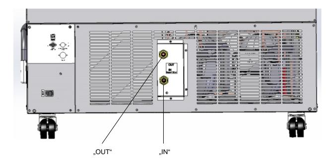
Figure 19: Connections of cooling water on the chamber rear (chambers with water cooling), example UF V 700  $\,$
