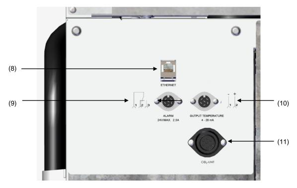
Figure 12: Connection panel (I) on the chamber rear
