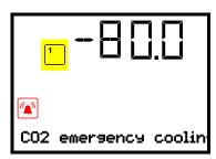
Normal display with running emergency cooling, showing the alarm message "CO2 emergency cooling"
