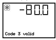
Normal display following the entry of a valid access code (example: code no. 3).
