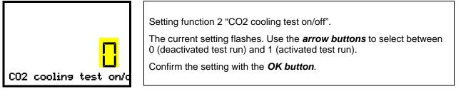
With the *Back button* you can go back to the "Functions on/off" submenu and, repeatedly pressing it, to Normal display.
