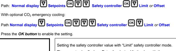
The current value flashes. Enter the desired limit value with the *arrow buttons*.
