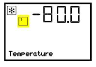
Normal display with activated emergency cooling
