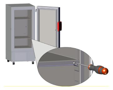
Figure 17: Inserting the shelf holders
