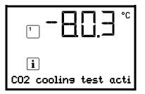
Information message (example:  $CO_2$  emergency cooling test run is active)
