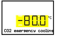
Setting the CO<sub>2</sub> emergency cooling temperature setpoint The current setting flashes. Enter the desired set-point with the arrow buttons. Setting range: -30 °C up to -90 °C Confirm the entry with the **OK button**..
