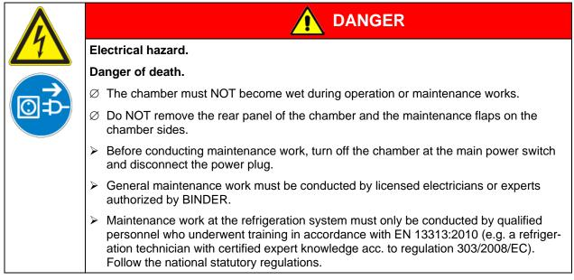
Ensure regular maintenance work is performed at least once a year and that the legal requirements are met regarding the qualifications of service personnel, scope of testing and documentation. All work on the refrigeration system (repairs, inspections) must be documented.
