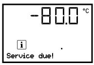
The message "Service due!" is shown in the text field of the controller display.
