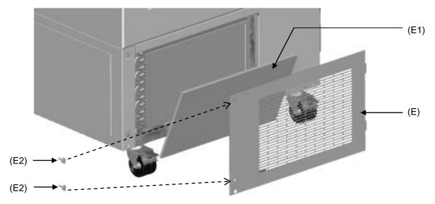
Figure 27: Removing the condenser air filter
