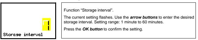
With the *Back button* you can go back to the "Data recorder" submenu and, repeatedly pressing it, to Normal display.
